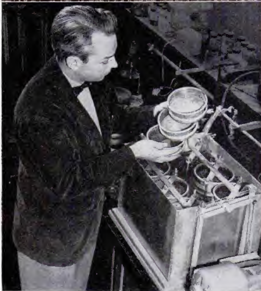
Dr. David Mowry, codiscoverer of Krilium, and the wet-sieving machine that tested 5000 combinations of soil and chemicals. Treated soil is put on sieves and sloshed up and down in water to test its stability
